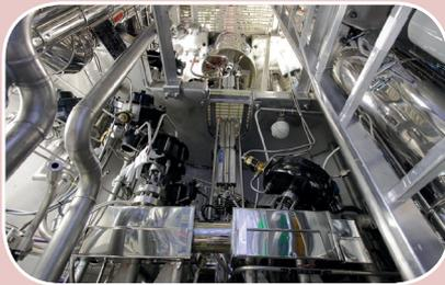
The CIP experimental program, led by the IRSN under the aegis of the OECD, includes a total of 10 tests. It consists of exposing fuel sections irradiated in the reactor to thermal-hydraulic conditions and the neutron power encountered during a reactivity injection accident.
