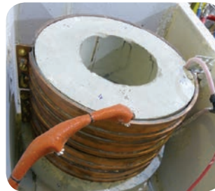
→ Concrete test section from the VULCANO facility
