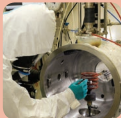
→ Installing a test component on VITI
